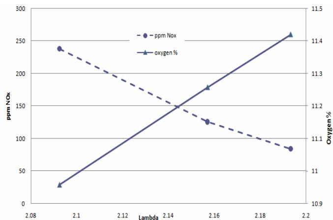
**FIG. 12 – EMISSION LEVELS FOR TWO-STAGE PRECOMBUSTION CHAMBER w/ePCC & PPC SPARK PLUG**
