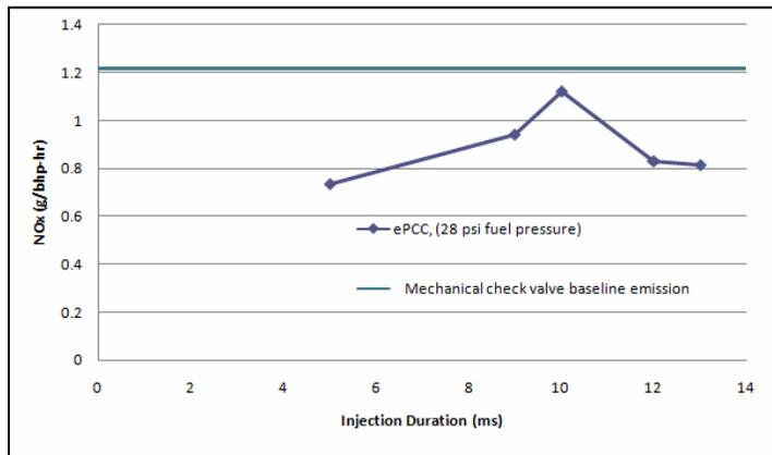
FIG. 8 – NOx PRODUCTION w/ELECTRONIC FUEL VALVE vs. BASELINE
