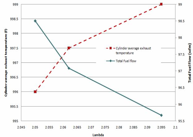
FIG. 9 – EGT & FUEL FLOW vs. LAMBDA w/ePCC
