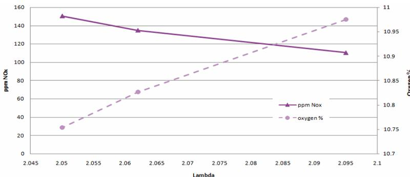
FIG. 10 – EMISSION LEVELS vs. LAMBDA w/ePCC
