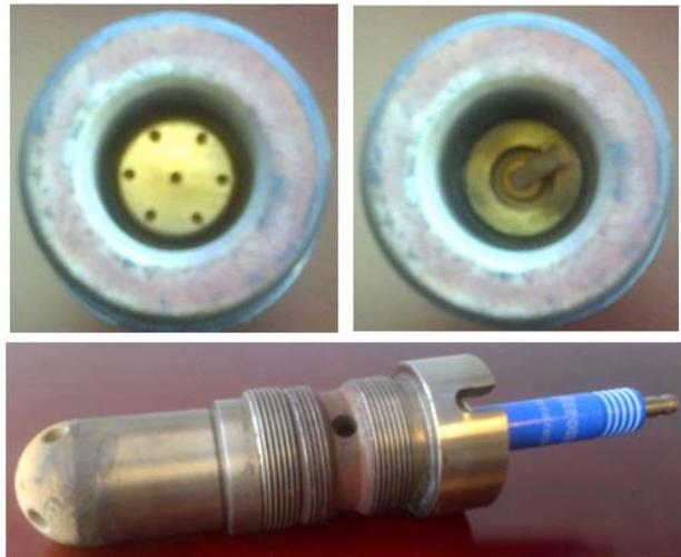
**FIG. 11 – PRE-COMBUSTION CHAMBER ASSEMBLY – PRE-COMBUSTION CHAMBER w/J-GAP SPARK PLUG (top right) – TWO-STAGE PRE-COMBUSTION CHAMBER w/PPC SPARK PLUG (top left)**
