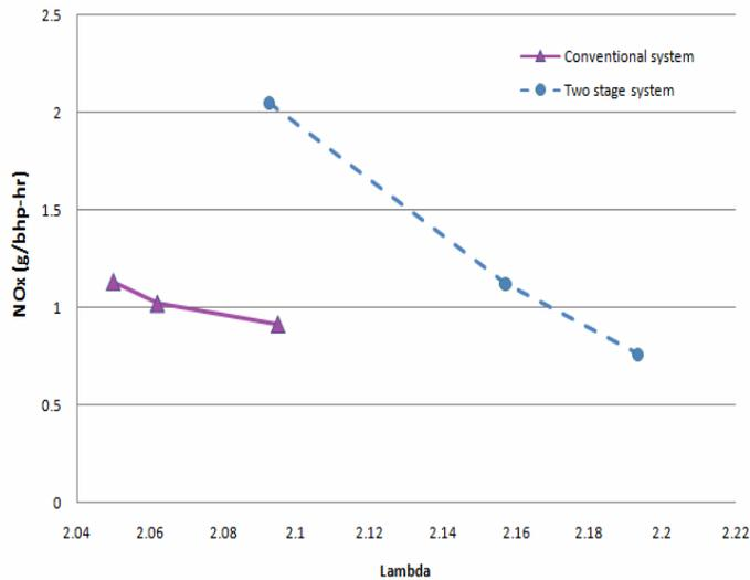
**FIG. 13 – NOx COMPARISON BETWEEN CONVENTIONAL PRE-COMBUSTION CHAMBER AND A NON-OPTIMIZED TWO-STAGE PRE-COMBUSTION CHAMBER w/ PPC SPARK PLUG**
