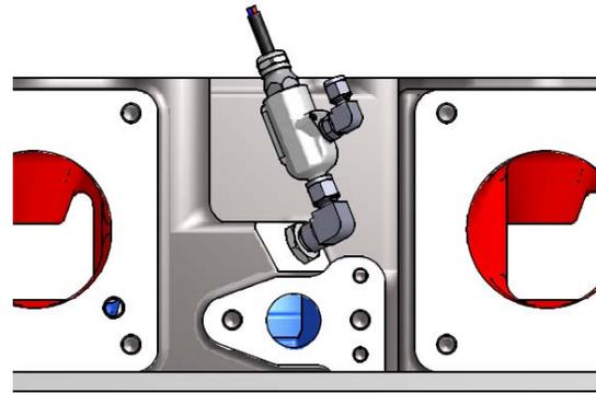
FIG. 2 – PRE-CHAMBER FUEL VALVE IN 6GTLX CYLINDER HEAD
